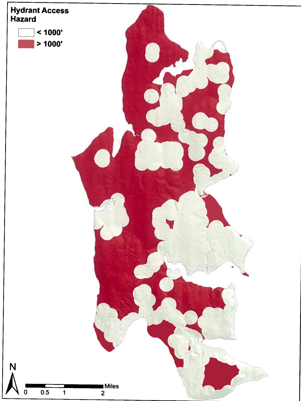
Figure 23: Hazard levels for the Hydrant Proximity factor.
